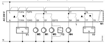
Basic connections for plant types with 2-position control (boiler with a 2-stage burner)
